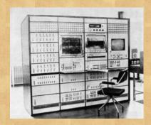
**Hybrid computers:** These types of computers are a combination of both Analog and Digital computers. The Digital computers are too slow and incapable of large mathematical operation. In hybrid types of computers the digital counterparts convert the analog signals to perform Robotics and Process control.
