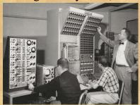
**Analog Computers:** It is different from a digital computer in respect that it can perform numerous mathematical operations simultaneously. It is distinct in terms of operation as it utilizes continuous variables for the purpose of mathematical computation. It utilizes mechanical, hydraulic, or electrical energy or operation.
