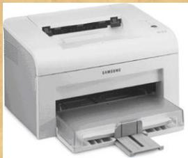
It is a high speed printer, uses laser technology. Laser recreates the image on a negatively charged drum, which attacks positively charged ink to the area image.
