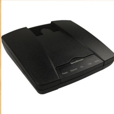
Modem is both an output and input device. Its full form is modulation and demodulation. It is an electronic device which helps the user to connect with the internet. The role of modem in a computer is to convert the analog signals to digital signals which a computer recognizes.
