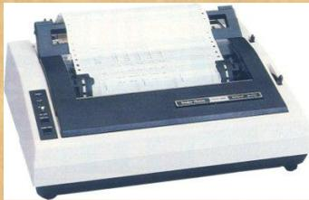
Impact printers are similar to an automatic typewriter, with a key striking an inked impression on paper for each printed character. The *Dot-Matrix Printer* (DMP) is a popular low-cost personal computer printer. It is an impact printer that strikes the paper one line at a time. It is still found in ATMs, small Point of Sale (POS) printers.
