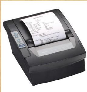
It uses heated pins to print images. On sensitive paper the pins are electrically heated and brought in to contact with concerned paper. When it is heated the coating on the paper discolors.
