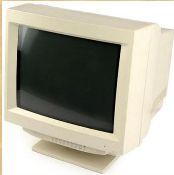
The CRT monitor creates a picture out of many rows or lines of tiny coloured dots. The CRT monitor comes in 15-inch to 21-inch sizes (38-53 cm) and larger though the actual viewing screen is about 1 inch (2.5 cm) smaller than the rated size.
