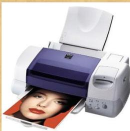
The best-known non-impact printer is the *inkjet* printer. The inkjet sprays ink from an ink cartridge at very close range to the paper as it rolls by.
