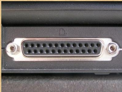
A port is an outlet on an equipment to which a plug or cable can be connected. *I/O ports* (Input/Output ports) are the interfaces to communicate with external devices such as printers, modems, joysticks, and terminals. Inputs are the received signals and outputs are the sent signals.
