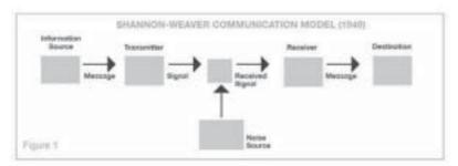
various concepts like Information source, transmitter, Noise, channel, message, receiver, channel, information destination, encode and decode.
