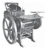
printing text from its invention by Johannes Gutenberg in the mid-15th century. In addition to the direct impression of inked movable type onto paper or another receptive surface, letterpress is also the direct impression of inked printmaking blocks such as photo-etched zinc "cuts" (plates), linoleum blocks, wood engravings, etc., using such a press.
